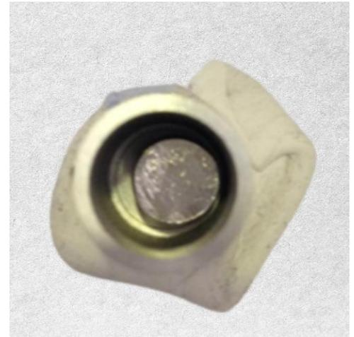
Figure 9 Ti in W crucible after deposition at 160W
