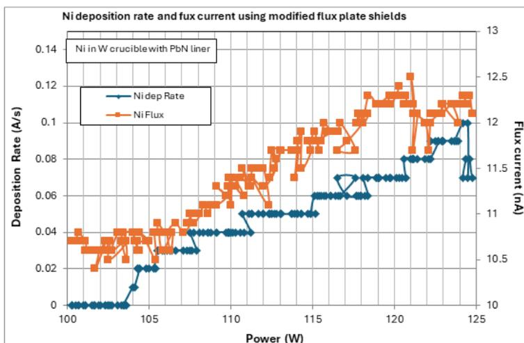
Figure 3 Deposition rate and Flux current for Ni in W crucible with PbN liner for a working distance of 100mm
