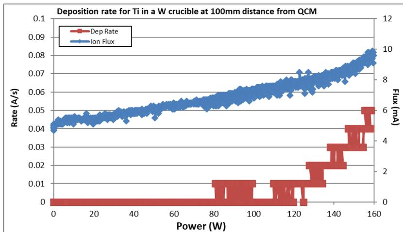
Figure 8 Deposition rate and Flux current for Ti in a W crucible
