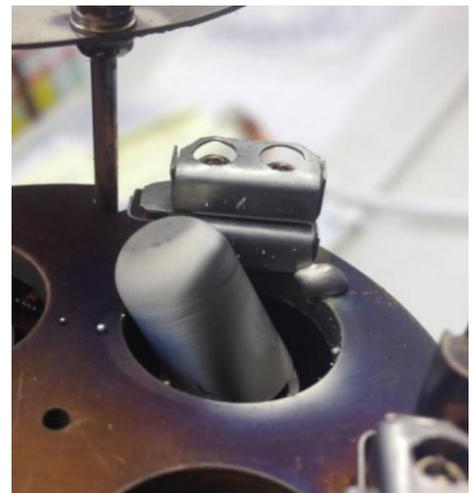
Figure 4 PbN liner popped out of W crucible at 125W
