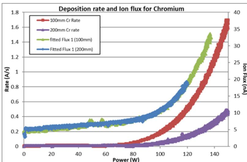
Figure 6 Deposition rate and Flux current for Cr in a W crucible
