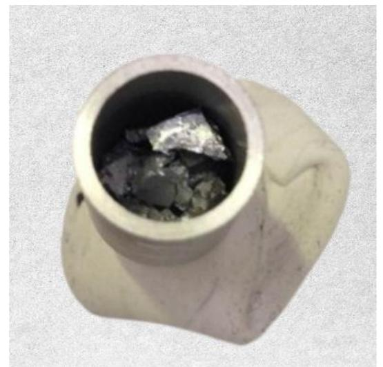
Figure 7 Cr in W crucible after deposition
