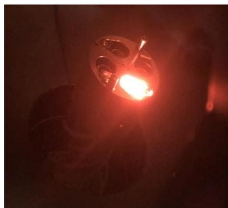
Figure 1 Evap-4 mounted inside the box chamber with pocket 3 powered up.
