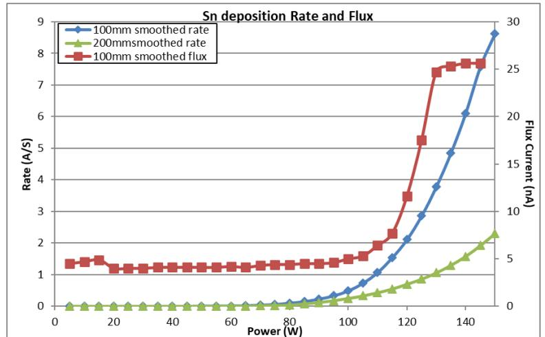
Figure 5 Deposition rate and flux current for Sn in a Ta crucible
