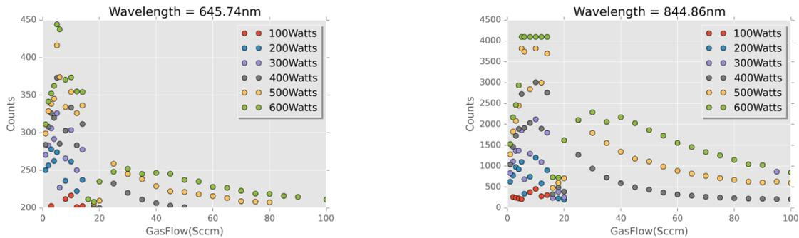
Figure 2 : Change in the intensity of the peak at 645nm (left) and 844nm (right) for Oxygen at different gas flows and power
