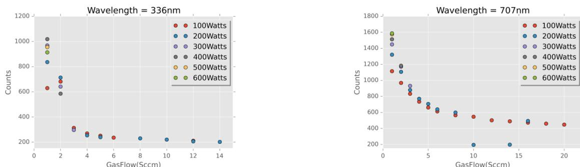
Figure 4 : Change in the intensity of the peak at 336nm (left) and 707nm (right) for Argon at different gas flows and power
