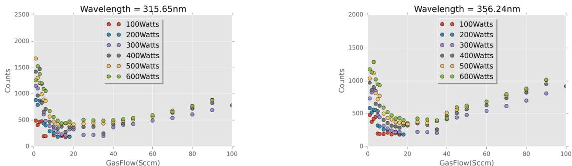
Figure 3 : Change in the intensity of the peak at 315nm (left) and 356nm (right) for Nitrogen at different gas flows and power
