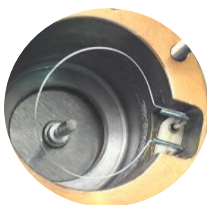
Figure 2 Evap-4 Pocket 2 loaded with the W rod and circular filament
