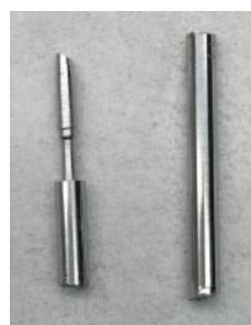
Figure 1 Shaped Tungsten rod (left) and standard Tungsten rod (right)
