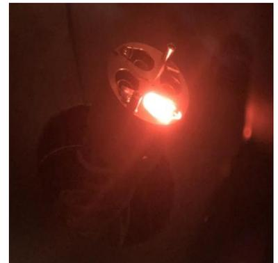
Figure 1 Evap-4 mounted inside the box chamber with pocket 3 powered up.
