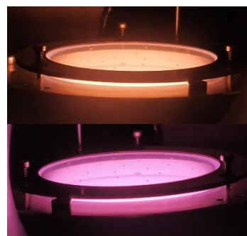
Figure 1 Operation of NL-ATS60 with N 2 RF plasma (top) and H 2 RF plasma (bottom)
